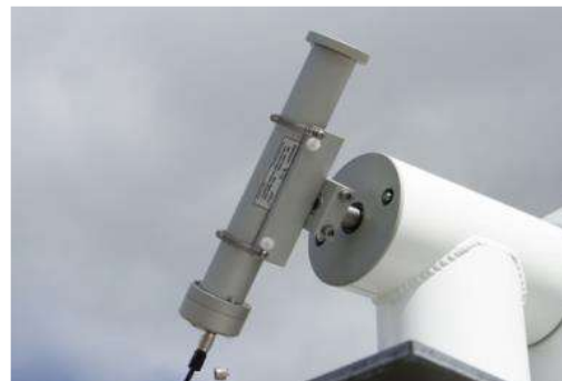
Solar radiation measuring unit
